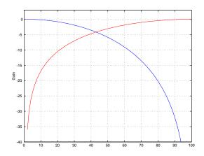
Figure 9.147: The gains applied to the mid cardioid (blue) and the side bidirectional (red) required to maintain a constant on-axis sensitivity for the virtual microphone as it rotates from  $0^{\circ}$  to  $90^{\circ}$ . Note that the x-axis of the graph does not directly correspond directly with any angle, however it is non-linearly related to the direction in which the virtual microphone is aimed.
