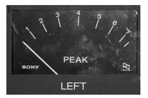
Figure 9.16: A photograph of a typical UK (or BBC) PPM on the output module of a Sony/MCI mixing console.
