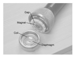
Figure 5.59: The same photograph as Figure 2a with the various parts labeled.
