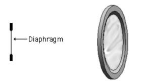
Figure 5.67: The construction of a diaphragm that's open on both sides.
