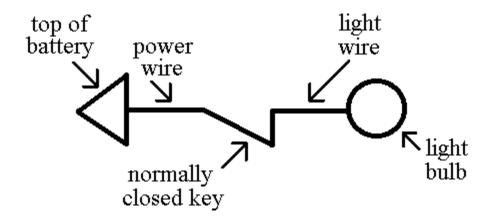
The picture and diagram at left show the top of a battery connected by a wire to a normally closed key, that is connected by another wire to a light bulb.
