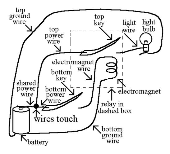
In this picture, only *one battery* powers all the circuitry in the previous picture. Note the symbol for wires that touch.
