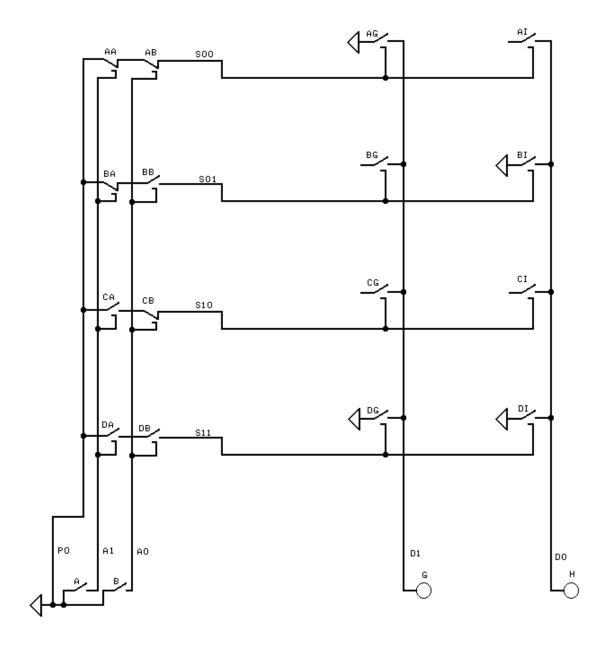
In the preceding circuit, keys A and B are the inputs and lights G and H are the outputs. The truth table for the circuit above is shown below.
