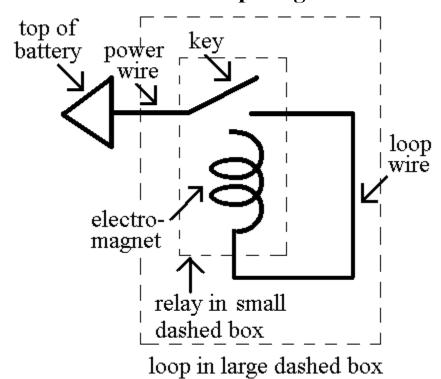
The picture and diagram at left show a relay that controls its *own* electromagnet! The square of wire that takes electricity from the key of the relay to the electromagnet of the same relay is called a 'loop.'
