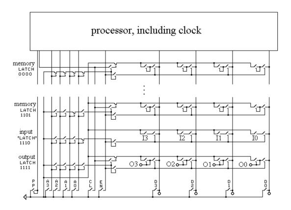
Inputs and outputs have been added to the computer above in place of two memory latches. When data is written to (copied to) 'output latch 1111,' then each loop, O3, O2, O1, and O0, will turn on its light if a 1 is stored in the loop. When data is read from (copied from) input 'latch' 1110 (It's not really a latch because it doesn't have loops.), then a 1 will be copied from key I3 if key I3 is pressed. If key 3 is *not* pressed, then a 0 is copied from I3. I2, I1, and I0 work similarly.
