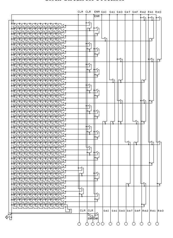
The preceding clock circuit shows a circuit that repeatedly generates the timing diagram signals. The outputs of this circuit can be connected to the processor to make the processor repeatedly execute instructions as indicated in the diagram of the complete (though simple) computer in the diagram below.
