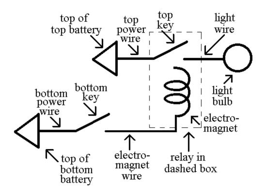
The diagram above shows the same circuit as the previous picture in a different way.
