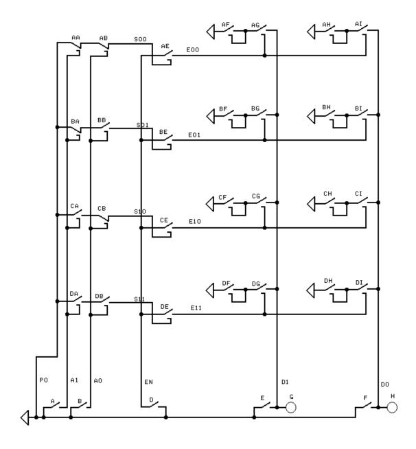
In the diagram at left, key E and key F (bottom right) have been added to the circuit. Keys E and F allow one to set a loop to value 1 without touching the loop's key.
