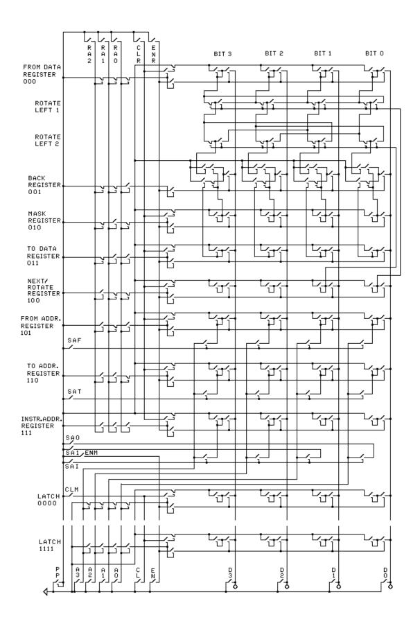
An instruction is executed in nine steps. Step 1 copies the address of the instruction from latch 0000 of the memory to the processor. Steps 2, 3, 4, and 5 copy the four words of the instruction to the processor. Step 6 copies the 'from data' to the processor. Step 7 copies the 'to data' to the processor. Step 8 copies the result from the processor to the memory. Step 9 copies the address of the next instruction to be executed from the processor to latch 0000 of the memory.
