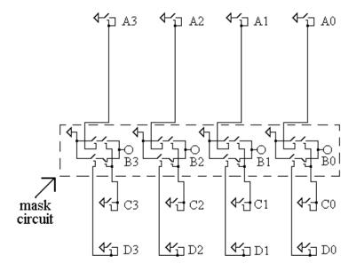
In the left circuit above, C3 controls whether the value of A3 or the value of D3 goes to B3. The other circuits behave similarly.
