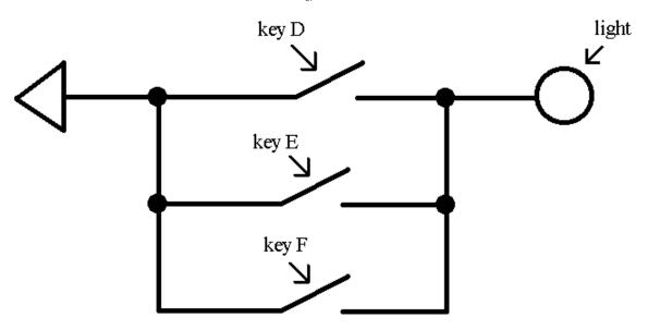
The light in the circuit above turns on when key D, key E, OR key F is pressed.
