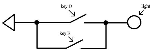
In the picture and diagram above, one need only press either 'key D' OR 'key E' (or both) to turn the light on.
