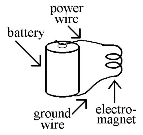
The picture above shows the top of a battery connected by a wire to an electromagnet.
