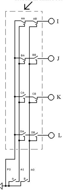
The diagram at left shows a 'decoder.' A and B are the inputs to the decoder and I, J, K, and L are the outputs. The truth table for this circuit is shown below.
