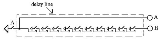
In the circuit (called a delay line) above, light B comes on ten hundredths of a second after light A. Ten hundredths of a second is one tenth of a second, so light B comes on one tenth of a second after key A is pressed (as indicated in the diagram below). (The small amount of time between the time key A is pressed and the time light A comes on is ignored.) Time 0 is 0 seconds and time 1 is one *tenth* of a second in the diagram below.
