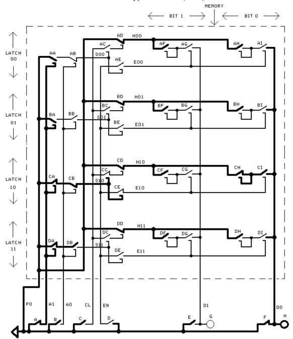
Step five: Keys A and F are released and address *wire* A0 and data *wire* D0 get value 0 (as indicated in the following diagram). Notice that *loop CH still has value 1*.
