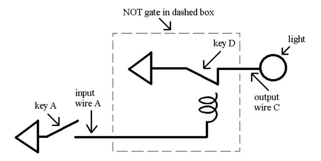
In the circuit above, the triangles are both the top of the *same* battery. When 'key A' is pressed, 'key D' is pulled down and the light goes *off*. That is, when 'key A' is pressed, normally closed 'key D' opens. Therefore, when 'key A' is pressed, the light goes *off*. Another way of describing the operation of the circuit is to say that 'output wire C' gets value 0 when 'input wire A' gets value 1. 'Output wire C' gets value 1 when 'input wire A' gets value 0.
