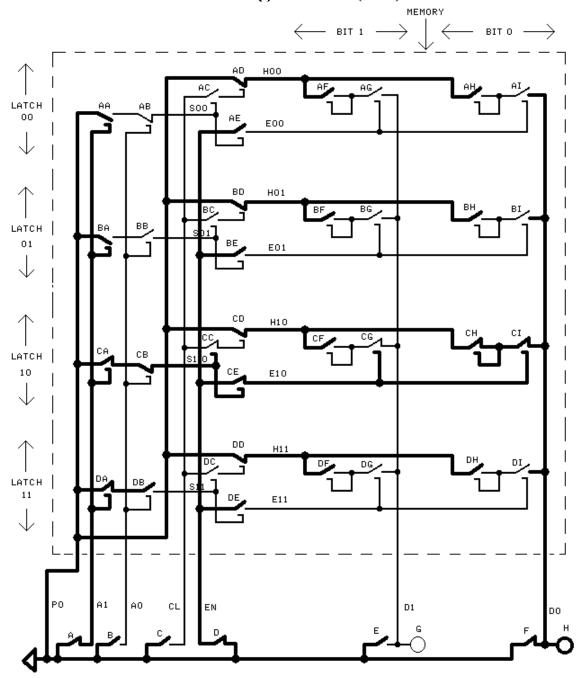
In the fourth step, key D is released and the enable (EN) wire returns to value 0 (unpowered). This results in power flowing through the memory as indicated by bold wires in the following diagram. Notice that loop CH still has value 1 even though loop CH is no longer connected to data wire D0 through relay CI (because relay CI is open).
