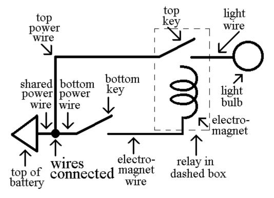
This diagram shows the same circuit as the previous picture in a different way. Touching wires are connected wires.
