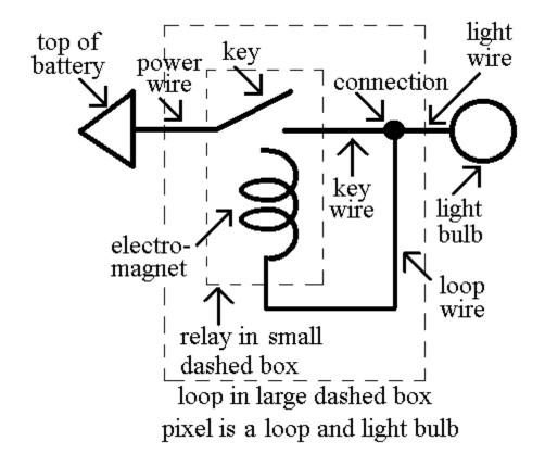
The picture and diagram above show a loop that controls a light bulb. A light bulb that is controlled by a loop is called a 'pixel.'
