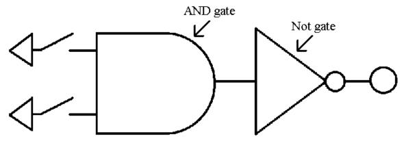
A 'NAND gate' can be constructed from an AND gate followed by a NOT gate as indicated below.
