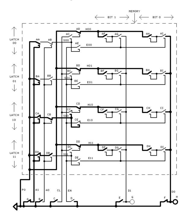
The *third* step in writing 01 to address 10 is pressing the enable key, 'D,' which controls the enable ('EN') wire. This results in power going through the circuit as indicated in bold in the following diagram. Notice that *loop* CH now has value 1. Loop CH got power from wire D0 through CI. *No* power went from wire D1 through CG to loop CF because wire D1 is *not* powered.
