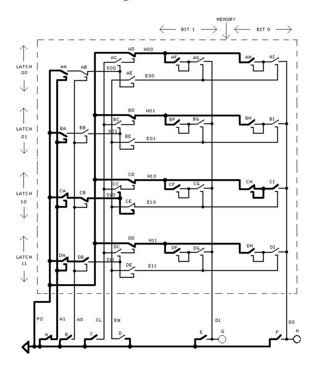
*Second*, press key D to make the enable (EN) wire have value 1. Then light H comes on indicating that bit 0 of latch 10 has value 1 and light G stays off indicating that latch 10 has value 0 in bit 1. This is shown in the following diagram.
