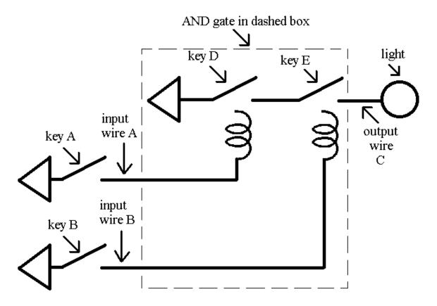
In the circuit above, the three triangles are all the top of the *same* battery. When 'key D' AND 'key E' close, then the light comes on. When 'key A' is pressed, then 'key D' closes. When 'key B' is pressed, then 'key E' closes. Therefore, when 'key A' and 'key B' are pressed, the light turns on. Another way of describing the operation of the circuit is to say that 'output wire C' gets value 1 only when 'input wire A' gets value 1 AND 'input wire B' gets value 1.
