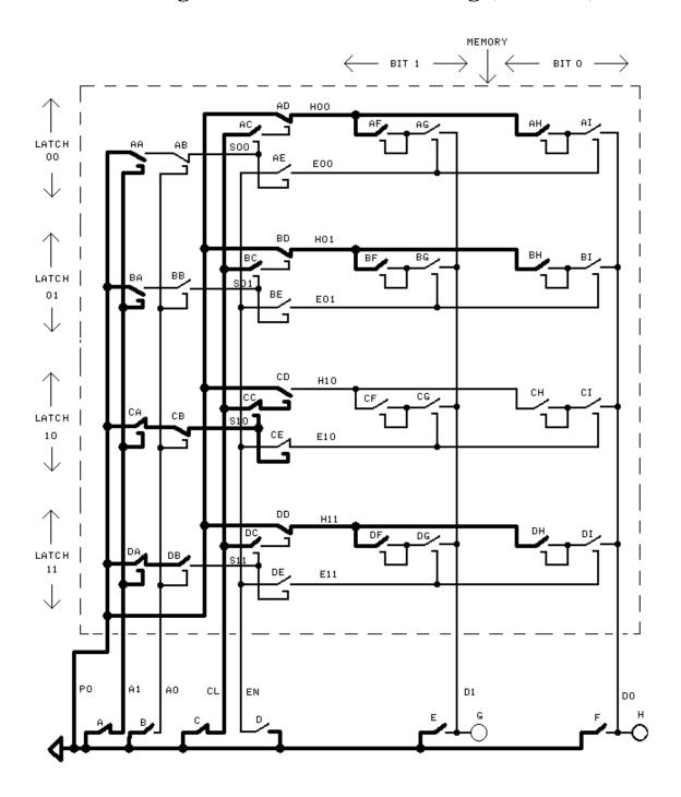
Release key CL after clearing latch 10 as indicated in the following diagram. Don't release key A until *after* CL is released so that you don't accidentally erase another latch.
