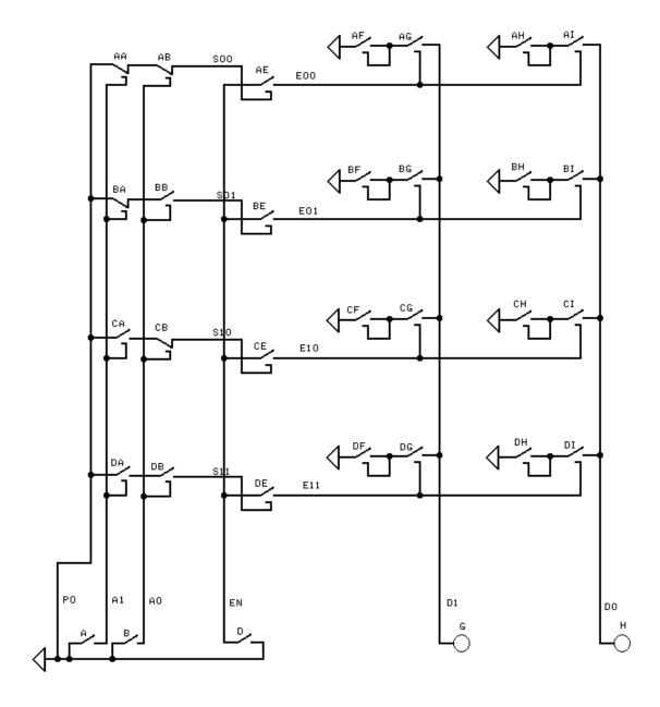
In the circuit above, eight loops have been added to the previous circuit. The loops are labeled AF, AH, BF, BH, CF, CH, DF, and DH. Each loop can have value 0 or 1. The truth table fore this circuit is shown below.
