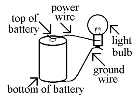
The picture above shows a 'battery' connected to a 'light bulb' by a 'power wire' and a 'ground wire.' A power wire is a wire connected directly to the top of the battery. A ground wire is a wire connected directly to the bottom of the battery. Any electrical machine is called a circuit.
