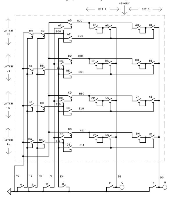
In this circuit, key C, wire CL (for CLear), relays AC, BC, CC, and DC, normally closed relays AD, BD, CD, and DD, and wires H00, H01, H10 and H11 (H for Hold, or remember) have been added to the circuit. These additions allow loops to be 'cleared' to value 0 by manipulating keys outside the dashed box (memory) without touching the loop keys.
