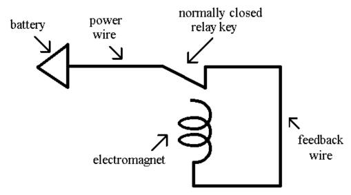
The picture and diagram at left show a normally closed relay that controls its *own* electromagnet. The square of wire that takes electricity from the normally closed key of the relay to the electromagnet of the same normally closed relay is called a feedback wire. (Notice that this circuit is different from a loop circuit, which uses a normally open relay.) This circuit is called an oscillator because the relay oscillates (changes back and forth) between open and closed.
