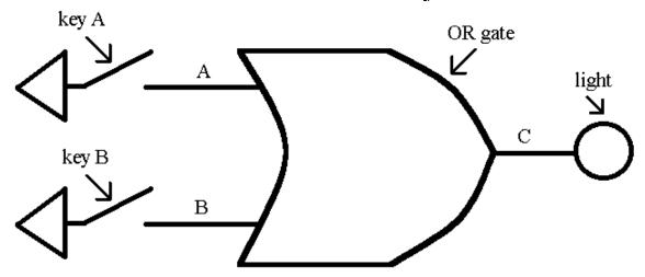
The diagram above shows a circuit with the symbol for an 'OR gate' which is shown alone, below.
