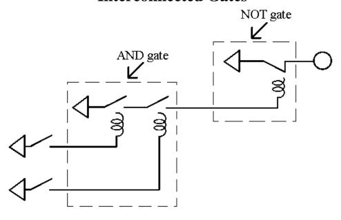
The diagram above shows that the output of an AND gate can be the input for a NOT gate. The circuit above can also be represented with gate symbols as below.
