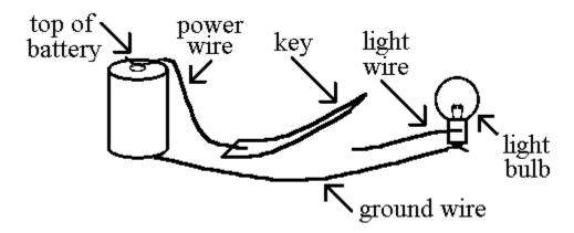
The picture above shows the 'top of' a 'battery' connected by a 'power wire' to a 'key' that is connected by a 'light wire' to a 'light bulb.'
