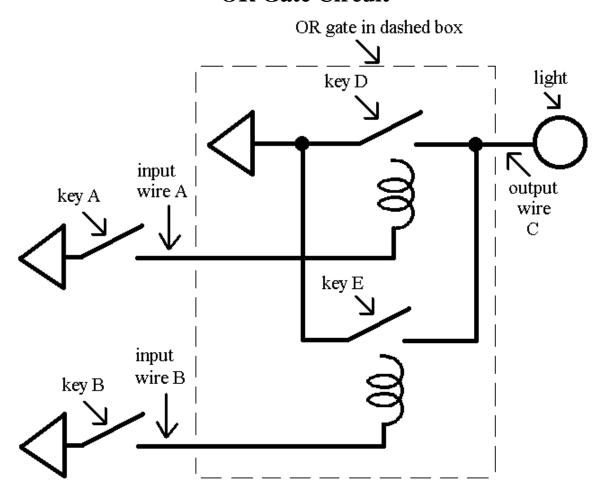
In the circuit above, as always, the *crossing wires do not touch* and are *not* connected to each other. When 'key D' OR 'key E' (or both) closes, the light comes on. When 'key A' is pressed, then 'key D' closes. When 'key B' is pressed, then 'key E' closes. Therefore, when 'key A' OR 'key B' is pressed, the light turns on. Another way of describing the operation of this circuit is to say that 'output wire C' gets value 1 only when 'input wire A' has value 1 OR 'input wire B' has value 1.
