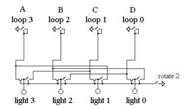
In the circuit above, if the 'rotate 2' key is *not* pressed, then loop 3 controls light 3, loop 2 controls light 2, loop 1 controls light 1, and loop 0 controls light 0.
