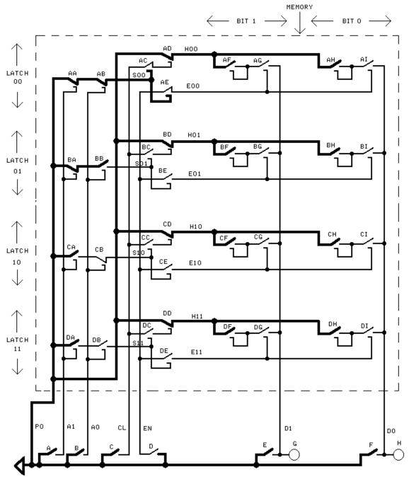
The **bold** wires in the diagram at left, show which wires are powered.
