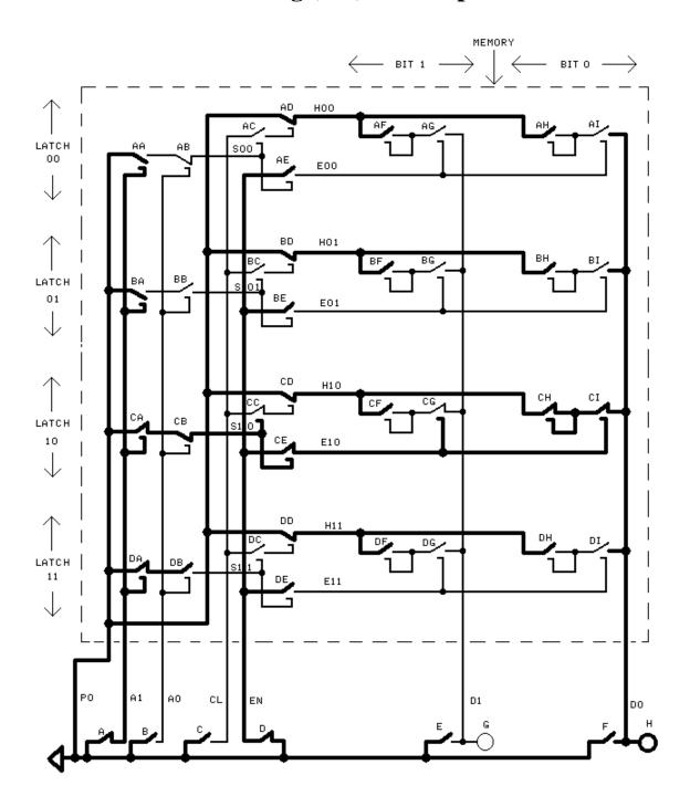
*Third*, release key D when done reading latch 10 (as indicated in the following diagram). That's all there is to reading a latch in memory.
