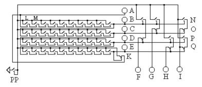
In the circuit above, key J in the upper left has been replaced by the normally closed relay K in the lower center of the circuit. The circuit above generates the timing diagram below when loop key PP in the lower left is pressed at time 0. Loop PP stays down after it is pressed.
