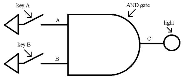
The diagram above shows a circuit with the symbol for an 'AND gate' which is shown, alone, below.
