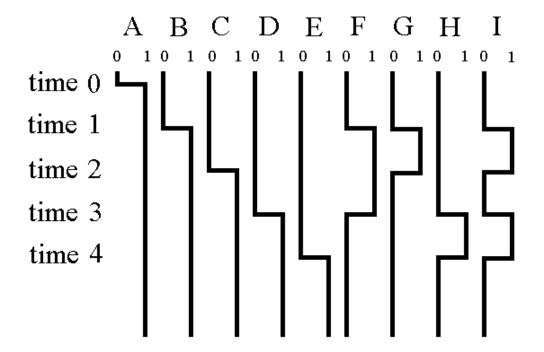
The timing diagram at left corresponds to the circuit above. Lights A, B, C, D, and E come on, in order, as before. However, the behaviors of lights F, G, H, and I are more complex.
