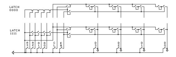
The circuit above shows a memory with four data wires (D3, D2, D1, and D0) and four address wires (A3, A2, A1, and A0). Because there are four address wires, there are sixteen possible latch addresses: 0000, 0001, 0010, 0011, 0100, 0101, 0110, 0111, 1000, 1001, 1010, 1011, 1100, 1101, 1110, and 1111. Only two latches, 0000 and 1111, are shown. The rest are implied by the gap in the circuit diagram.
