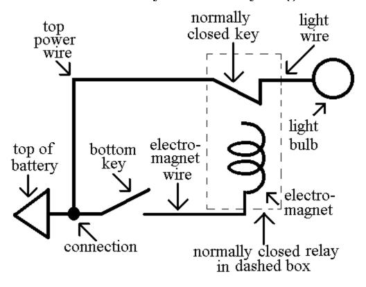
The preceding picture and diagram show a bottom key that controls an electromagnet. The *electromagnet*, in turn, controls the *top*, *normally closed key*. A normally closed key and the electromagnet that controls it are, *together*, called a normally closed relay.
