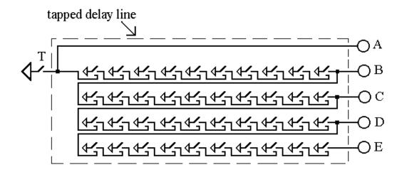
The circuit above is called a tapped delay line. Wires A, B, C, D, and E are called taps. Light B comes on one *tenth* of a second after light A, light C comes on two tenths of a second after light A, light D comes on three tenths of a second after light A, and light E comes on four tenths of a second after light A (as indicated in the timing diagram below).
