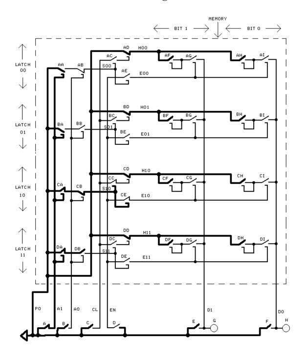
The memory in the drawings is very small. There are only two address wires and two data wires. Because there are two address wires, there are four possible addresses: 00, 01, 10, and 11, and, so, four latches. Because there are two data wires, each latch has two loops. Each loop holds one 'bit' of information, a 0 or a 1. Four latches with two loops each means  $8 (= 4 \times 2)$  loops total.
