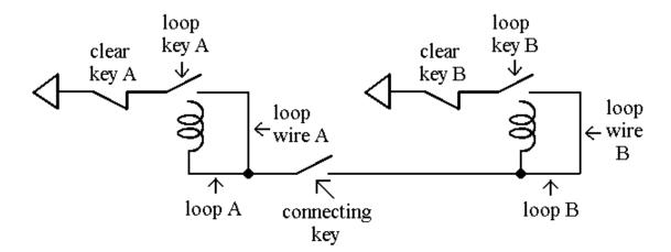
In the circuit above, the 'connecting key' connects loop A and loop B. Both loops have value 0. Temporarily pressing 'loop key A' gives the value 1 to loop A. Now, temporarily pressing the 'connecting key' will make loop B have value 1. That is because when loop A has value 1, loop key A is closed, loop wire A has value 1, and when the connecting key is closed, electricity can reach the electromagnet of loop B, giving loop B value 1.
