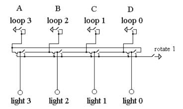
In the circuit above, if the 'rotate 1' key is *not* pressed, then loop3 controls light 3, loop 2 controls light 2, loop 1 controls light 1, and loop 0 controls light 0.
