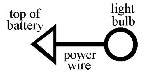
The diagram above also shows a 'battery' connected to a 'light bulb' by a 'power wire' and a 'ground wire.' This *diagram* means the same as the picture on page 2. *The ground wire is not shown* because it is assumed that one connection of every light is always connected to the bottom of the battery by a ground wire *in diagrams*. Diagrams are simpler to draw than pictures that mean the same thing.
