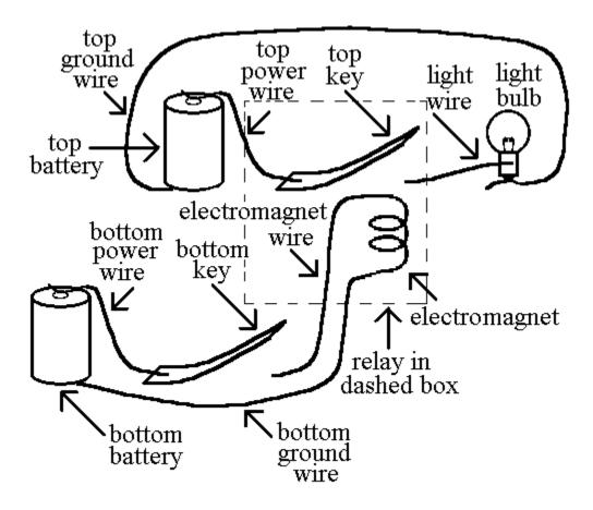
The picture above shows a 'bottom key' that controls an electromagnet.
