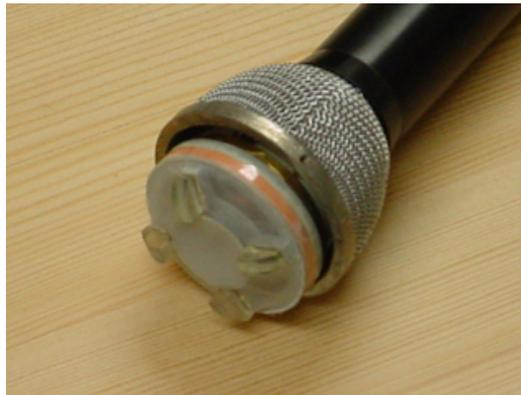
Figure 5.57: A moving coil dynamic microphone with the protection grid removed. The “front” of the microphone shows a second protective layer made of mesh and hard plastic. The diaphragm and assembly are below this.
