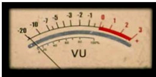
Figure 9.13: A typical Type A VU Meter on a Joe Meek compressor.
