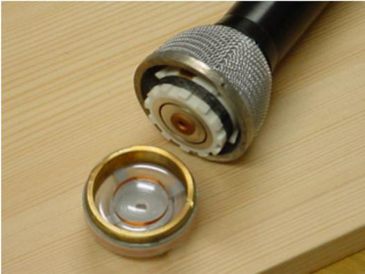
Figure 5.58: The underside of the diaphragm showing the copper coil glued to the back of the diaphragm. This coil fits inside the circular gap in the magnet. See Figure 3a for part labels.
