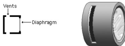
**Figure 5.74:** A microphone that is one half pressure transducer and one half pressure gradient design. Note that if you build this microphone it probably will not work properly – this is an approximate drawing for conceptual purposes. The significant things to note here are the vents that allow some of the pressure changes from the outside world into the back of the diaphragm. Note, however, that the back of the diaphragm is not completely exposed to the outside world.
