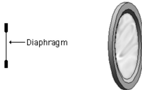
Figure 5.67: The construction of a diaphragm that's open on both sides.
