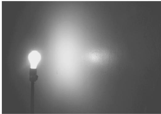
**Figure 3.19:** Photograph of a wall surface which exhibits both specular and diffusive reflective properties. Note that there are two bright spots. The small area on the right is the specular reflection, the larger area in the centre is the diffuse component.
