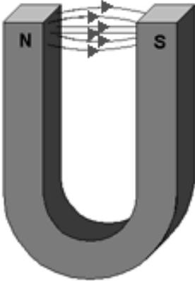
Figure 2.23: Magnetic lines of force around a horseshoe magnet.
